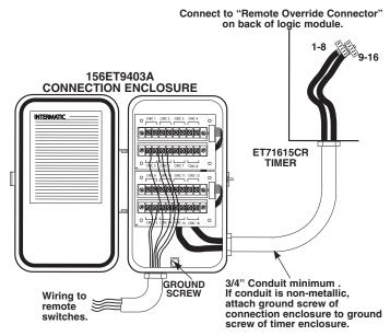
This accessory allows for the connection of up to 16 remote override circuits to Intermatic ET71615CR series timers. See instruction manual for function and programming information.
